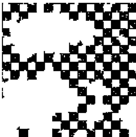
FIG. 11. A particular realization of the 8 \times 8 checkerboard lattice at its critical point p_{c,n}=0.642318 (as given in Table I), showing in black the sites wetted by the largest cluster. The total lattice is 128 \times 128 sites, with periodic boundary conditions.
